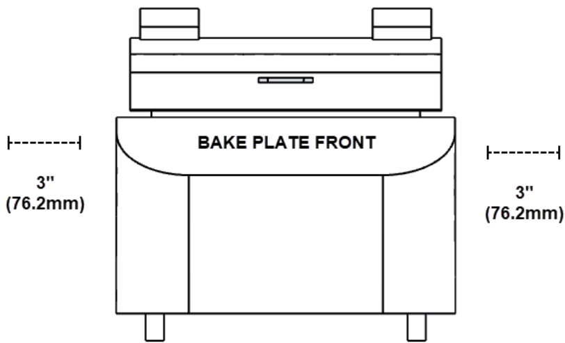
Figure 2: Apogee® 300 Bake Plate Side Clearance Requirements
